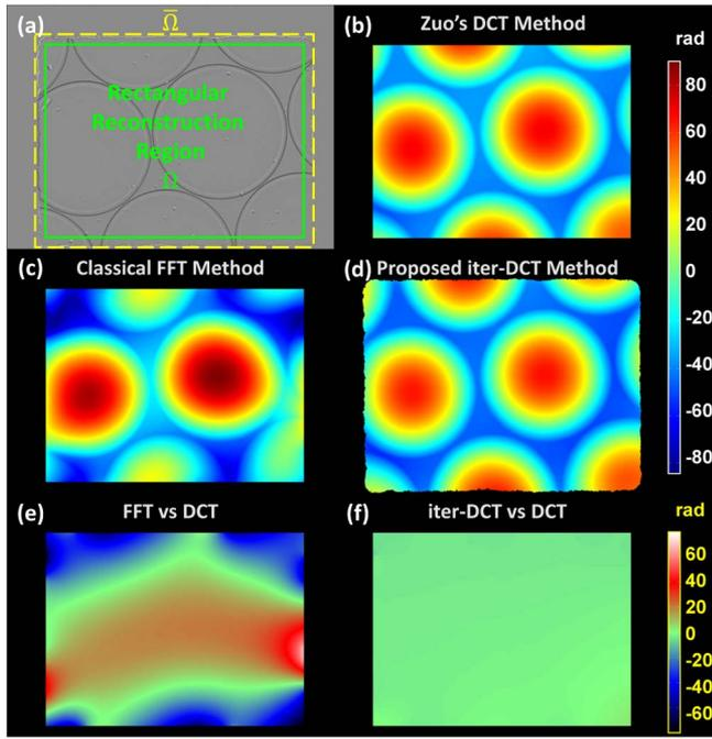
Fig. 8. Zuo's DCT method uses the information in "data region  $\tilde{\Omega}$ " to retrieve phase in reconstruct region  $\Omega$  (a), and its result (b) is used as a benchmark to judge the results from classical FFT-based TIE solver (c) and the result from the proposed iter-DCT method (d). The phase retrieved with the proposed method is much closer to the DCT result (f) than the FFT one is (e).
