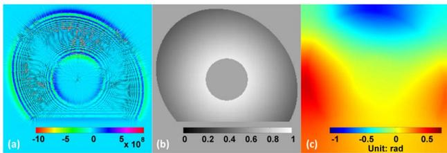
Fig. 4. With the inputs of the calculated  $J$  (a) and filled intensity (b), the DCT-based TIE solver can estimate an initial phase (c).
