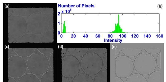
Fig. 7. Experimentally captured intensity at focus (a) with its histogram (b), and the intensity at  $-550$   $\mu$ m (c) and  $+550$   $\mu$ m (d) as well as their intensity derivative  $dI/dz$  (e).
