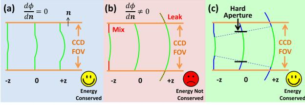
Fig. 1. Energy conservation is required in TIE. (a) Energy is conserved when phase derivatives in the normal directions at boundary edges  $d\phi/dn = 0$ . (b) Energy is not conserved when  $d\phi/dn \neq 0$ . (c) A hard aperture is added in the optical wavefield to make sure of the energy conservation.
