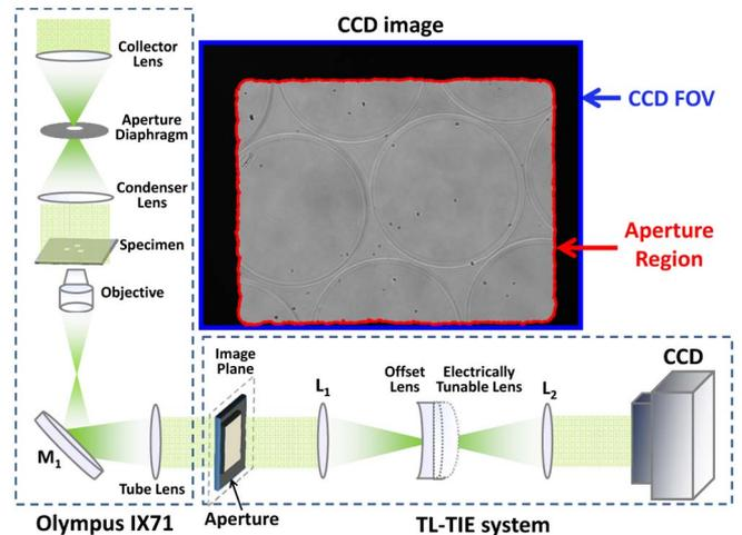
Fig. 6. TIE experiment is implemented by using an inverted bright-field microscope and a tunable lens-based TIE module with placing an aperture at the image plane.
